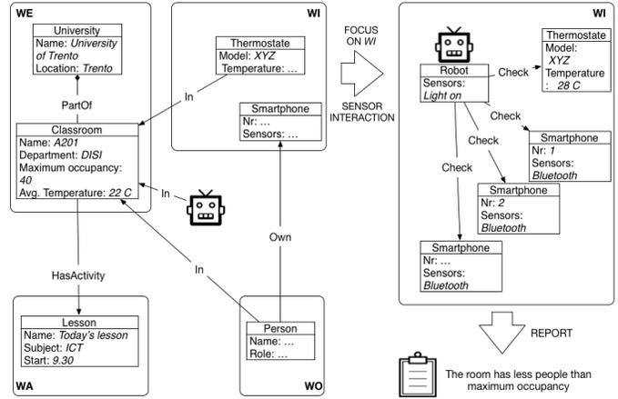
Fig. 3. The case of occupancy as a knowledge graph, showing our sensing system coupled with the enduring context model.
